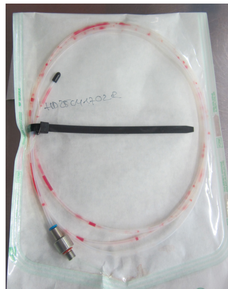
Fig. 1. Test tube after standardized contamination.
