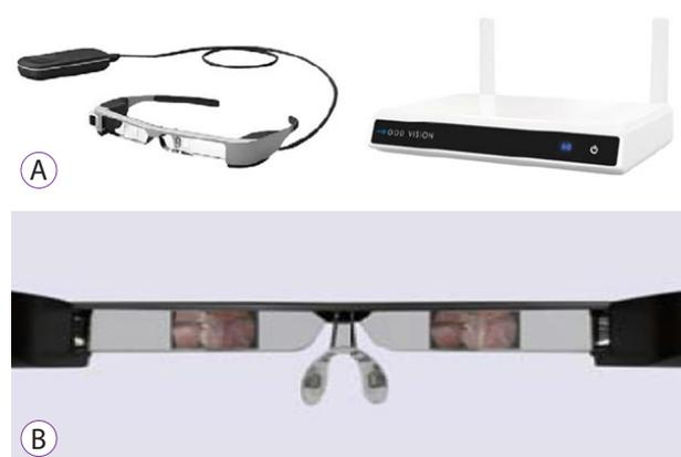
**Fig. 1.** (A) Components of the wearable display glasses, including smart glass, a controller, and the main unit module. (B) Wearer's view.
